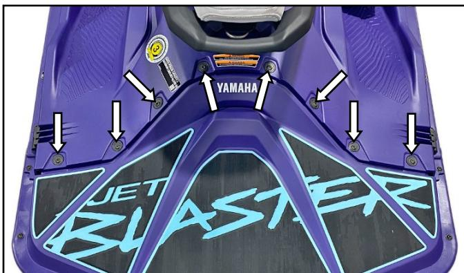
Remove bolts & nuts (9 each side) securing main deck to hull.
