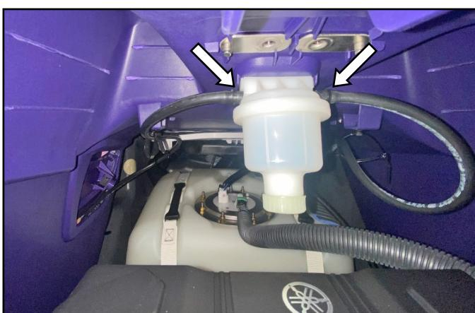
With assistance, carefully lift main deck at sides and remove towards rear of craft. **NOTE: Be sure to support glove box during and after removal of main deck.**
